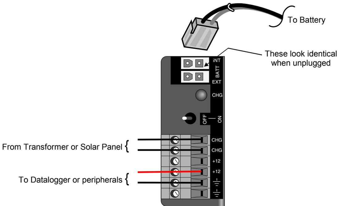
FIGURE 1. Wiring to Charger
