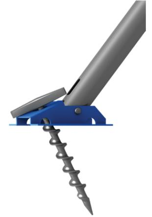
Place the tip of an anchor through the hole in the top of the foot. Turn the handle clockwise, applying downward pressure, until the anchor fully secures the tripod foot to the ground.
