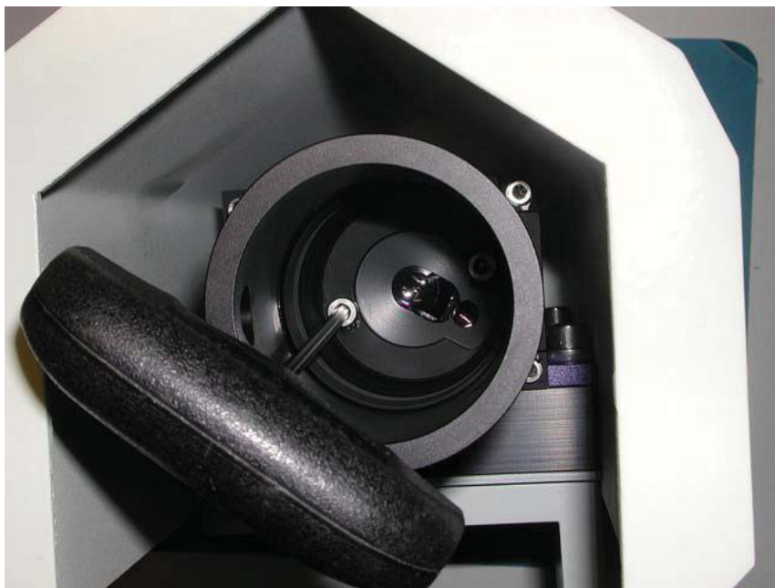
Figure 7-1 Unscrew the tube for stray light reduction to clean the mechanics and optics.
