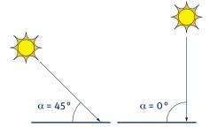
Ideally a pyranometer has a directional response which is exactly the same as the cosine-law. However, in a pyranometer the directional response is influenced by the detector and by the quality, dimensions and construction of the dome(s). The maximum deviation from the ideal cosine-response of the pyranometer is given up to 80° angle of incidence with respect to 1000 W/m² irradiance at normal incidence (0° zenith angle).
