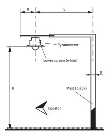
As a guide, a black shadow below the pyranometer with a radius of 0.1 x H decreases the signal by 1%, and 99% of the signal will originate from an area with a radius of 10 x H.
