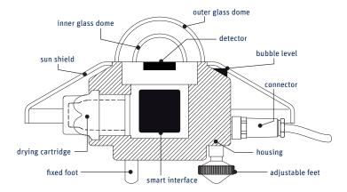
A drying cartridge in the SMP11 radiometer housing is filled with replaceable silica gel and prevents condensation on the inner sides of the domes, which can cool down considerably on clear windless nights. The SMP3 has a sealed construction with a non-replaceable internal drying cartridge. The SMP10 has an internal desiccant that lasts for 10 years.
