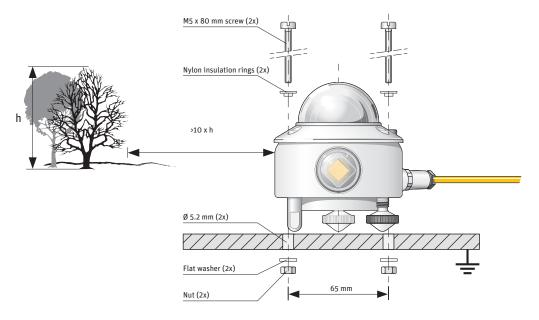
Note After recalibration and/or reinstallation ensure that the nylon insulators are refitted.
