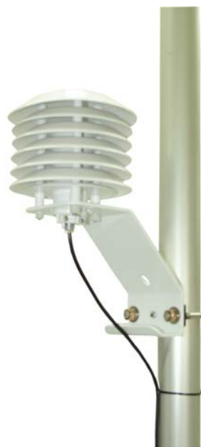
FIGURE 3.2. HMP60 and 41303-5A Radiation Shield on a Tripod Mast
