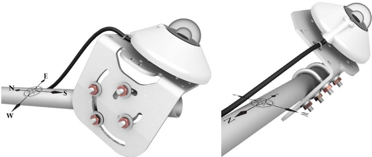
FIGURE 7-3. Two views of a pyranometer mounted at an angle for the Northern Hemisphere
