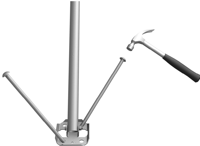
FIGURE 1.5-7. Staking the Tripod Feet
