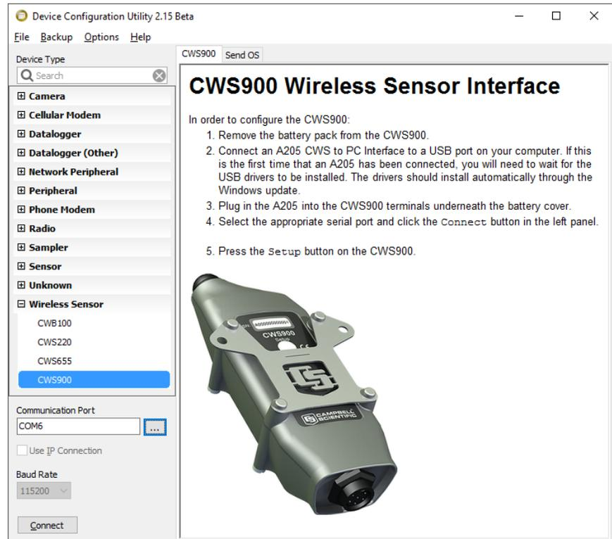
Once *Device Configuration Utility* connects to the sensor, enter the address of the CWB100 in the **Base Station Address** field. If configuring a CWS900, select the type of measurement the sensor will make from the **Measurement Configuration** list. If desired, change the **Sensor Name** from its default value.
