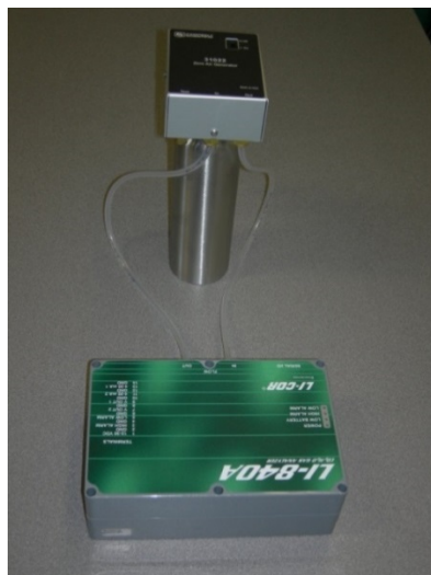
FIGURE 6-5. Zero Air Generator connected to LI-840A
