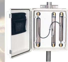
The CPEC200 Scrub Module is an accessory to the CPEC200. It is used to provide a source of zero air for zeroing the EC155 CO<sub>2</sub>/H<sub>2</sub>O analyzer. It uses a small, low-power (2W) diaphragm pump that is mounted in a temperature-controlled and weathertight fiberglass enclosure. Ambient air is drawn through molecular sieve to remove CO<sub>2</sub> and water vapor, and push zero air to the EC155 at approximately 2 l-min<sup>-1</sup> flow.
