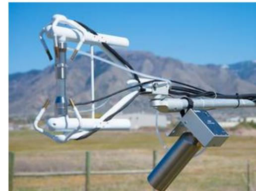
An accelerated usage test was performed at Campbell Scientific, Inc., from January to May, 2016. Open-path IRGAs (EC150 and IRGASON) were zero and spanned using traditional compressed gases and dewpoint generator, and then air from the Zero Air Generator was measured. The run time for the pump was recorded for each test.
