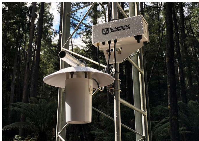
One of the AP200 intakes and the aspirated temperature probes
