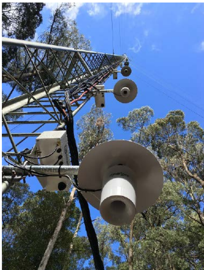
One of the AP200 intakes and the aspirated temperature probes
