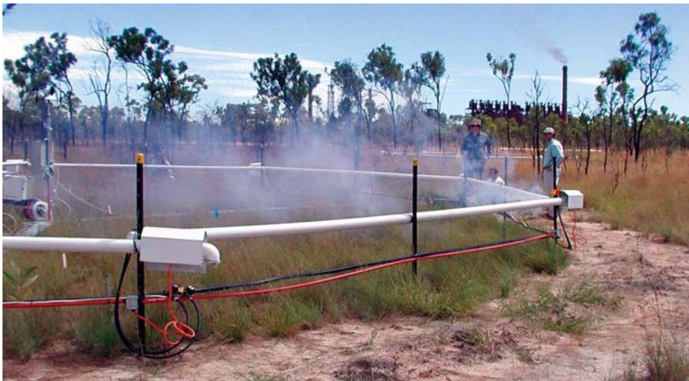
Testing the CO 2 delivery system with a smoke generator during the OzFace installation.
