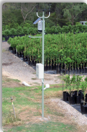
Tower Weather Station - fixed into ground for longterm use
