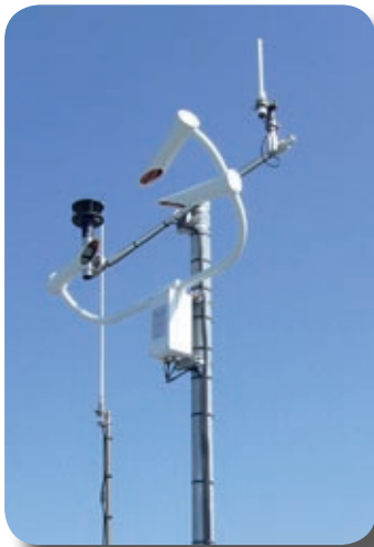
Six road weather stations have been installed to monitor the road during adverse conditions
