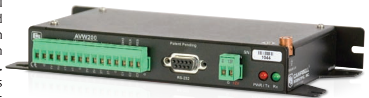
The AVW200 is an interface that eliminates the effects of external electromagnetic noise on vibrating-wire measurements.
