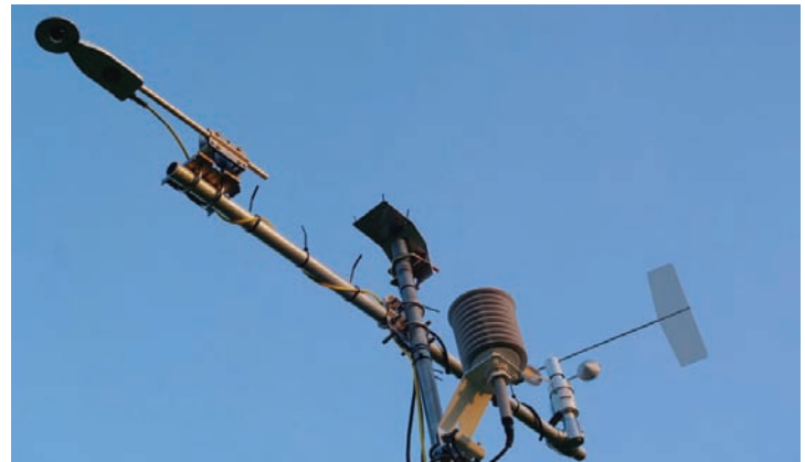
LW/SW/Net radiometer, PPFD, RH%, Airtemp, windspeed & winddirection on top. On the ground, not visible: heatflux, leaf wetness, TDR, soiltemp & averaging soil-temp. The zip-ties keep the birds away
