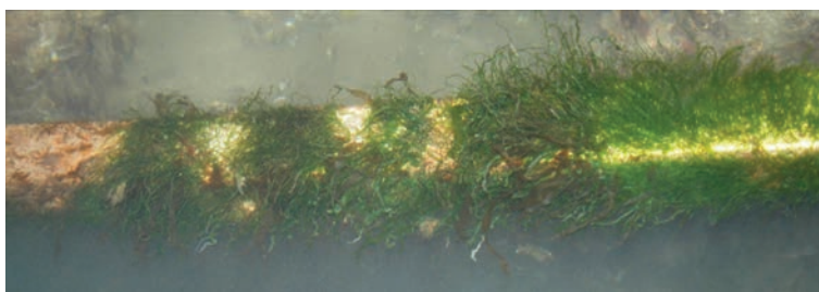
Above: The intake arm with growth after 6 weeks
