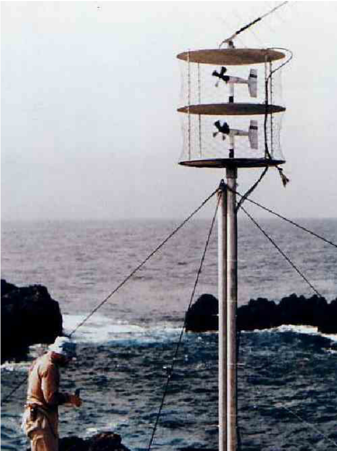
An innovative method of discouraging interference from birds was used at a station at St. Peter and St. Paul Rocks (Brazil). Photo courtesy Dr. Silvia L. Garzoli (Director of the Physical Oceanography Division of the Atlantic Oceanographic and Meteorological Laboratory of NOAA).
