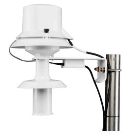
For the upper measurement, attach the 43502 to the top most mast of a UT20 or UT30 tower (20 ft and 30 ft measurement heights, respectively).
