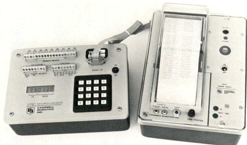
The CR56 Printer, shown above with the CR21, can be used to obtain on-line printed copy where environmental extremes or lack of AC power would limit the use of standard computer peripheral type printers.
