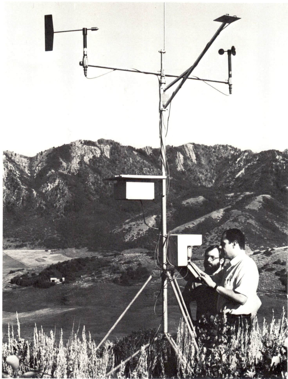
Complete station for monitoring wind speed, wind direction, solar radiation, air temperature, humidity, precipitation, and soil temperature.
