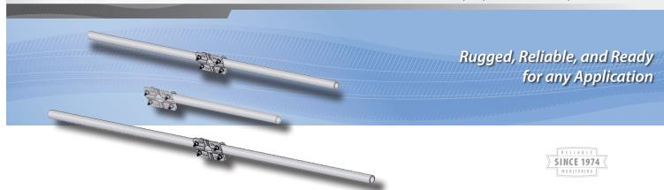
Crossarms provide a rugged attachment point for securing meteorological sensors, antennas, and other peripherals to our tripods and towers. They place sensors a few feet away from the midline of the tower or tripod, thereby serving to reduce the effects of the mount on the sensor measurement. Sensors or peripherals are mounted to the end of the crossarm using an appropriate mount (see General Mounts, Solar Radiation Mounts, and Solar Radiation Shields brochures).
