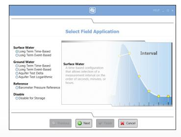
HydroSci software simplifies the process of configuring the sensor to monitor surface water, ground water, or a standard pump test.
