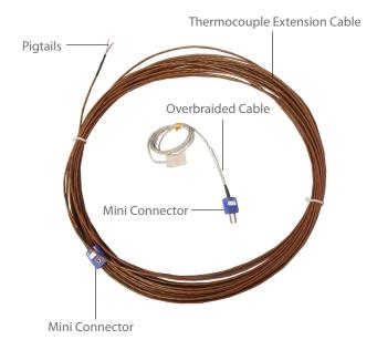
The CS220 is shipped with a stainless-steel overbraided cable and a thermocouple extension cable. The pigtails of the extension cable connect to the datalogger (see Wiring Table).
