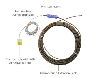
The mini connectors of the thermocouple extension and overbraided cables attach to each other (shown above). Adhesive under the masking paper secures the sensor to a solar panel.
