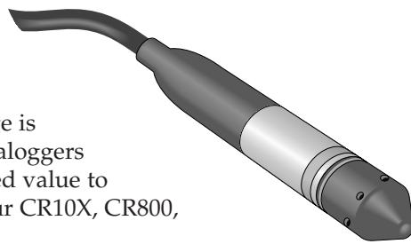
The CS420 and CS425 feature a titanium body, 0.69" outer diameter, isolated diaphragm, and a polyurethane cable. The cable is vented, which eliminates the need to compensate for changes in barometric pressure. This cable must terminate inside a desiccated enclosure or a Campbell Scientific DES2 desiccant case.
