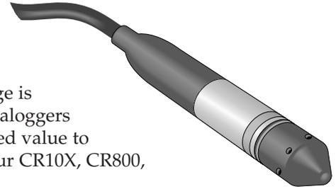
The CS420 and CS425 feature a titanium body, 0.69" outer diameter, isolated diaphragm, and a polyurethane cable. The cable is vented, which eliminates the need to compensate for changes in barometric pressure. This cable must terminate inside a desiccated enclosure or a Campbell Scientific DES2 desiccant case.
