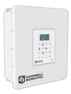
The CD100 has a vacuum fluorescent display for responsive use through a very wide operating temperature range. It has a water and dust ingress protection rating of IP66 when installed.
