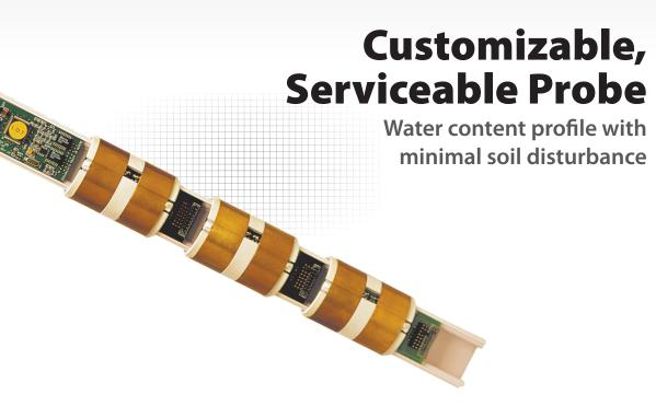
Water content profile with minimal soil disturbance
