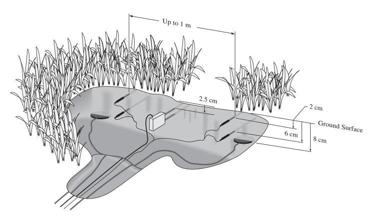
Above is an example energy-balance installation. The HFP01 Heat Flux Plates are installed with the CS616 Water Content Reflectometer and TCAV Averaging Soil Temperature Probes. All sensors must be completely inserted into the soil face before the hole is backfilled.
