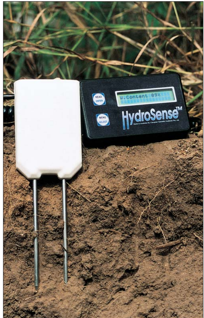
The Hydrosense system consists of the CS620 sensor (left), the CD620 display (right), and two rods.
