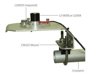
To attach the CM225 to a crossarm, place the U-bolt in the holes on the bottom of the bracket (shown). If the CM225 is attached to a mast, place the U-bolt in the holes in the side of the bracket.
