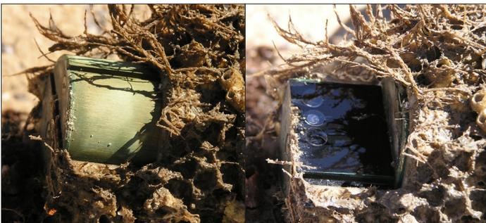
Biological fouling on a closed sensor (far left) and an opened sensor after 86 days of deployment in the Atlantic Ocean near Savannah, Georgia.
