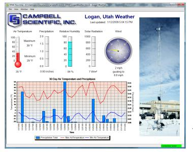
RTMC projects developed in RTMC Development or RTMC Pro are run using RTMC Run-Time. RTMC Run-Time is included with LoggerNet, LoggerNetAdmin, RTDAQ, and RTMC Pro. Additional RTMC Run-Time versions can be purchased separately and installed on computers that are networked to a LoggerNet computer. This allows remote computers to display data in a graphical format from a LoggerNet server.
