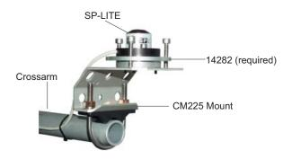
To attach the CM225 to a horizontal crossarm, place the u-bolt in the holes on the bottom of the bracket (shown). To attach the CM225 to a vertical mast or pole, place the u-bolt in the holes in the side of the bracket.
