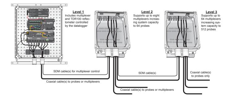
A complete TDR100-based system includes the TDR100, SDMX50-series multiplexers, dataloggers, power supplies, enclosures, and probes. Specifications and other information about the other components can be found in the *SDMX50-series Multiplexer* component category brochure, *TDR Probes* component category brochure, and *TDR100-Based* system brochure. These brochures are available at: <a href="http://www.campbellsci.com/product-literature">www.campbellsci.com/product-literature</a>
