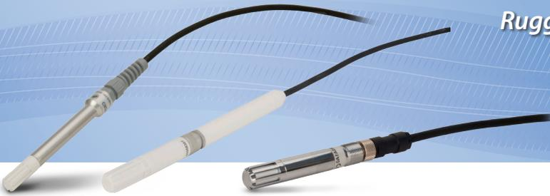
Air temperature and relative humidity probes typically consist of two separate sensors packaged in the same housing. Often relative humidity is measured with a capacitive RH chip, while air temperature is measured by a PRT. The HMP155A, HC2S3 or CS215 is recommended
