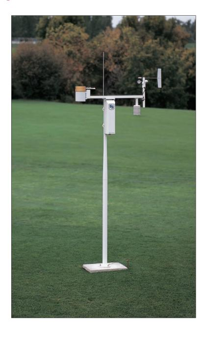
The T. Weather Station incorporates the Campbell Scientific CR10X Measurement and Control Module to measure sensors, process and store data, and communicate with the central computer. Simple specifications for the CR10X and sensors are listed on the back of this page.
