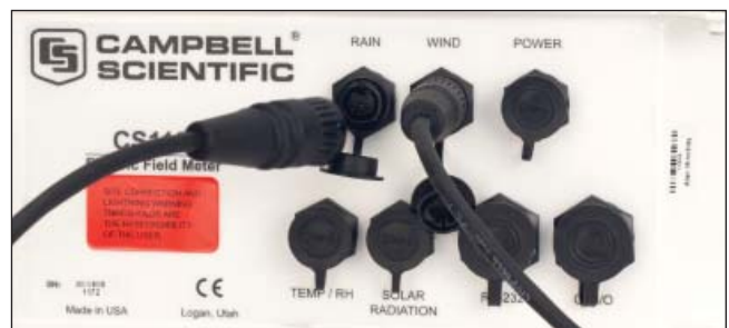
The WMS100 has field wiring options that simplify the attachment of sensors and down-tower cables.
