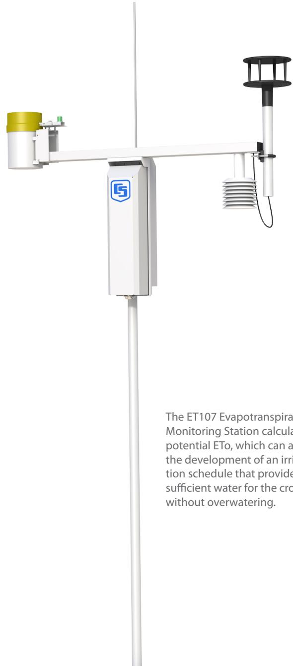
The ET107 Evapotranspiration Monitoring Station calculates potential ETo, which can aid in the development of an irrigation schedule that provides sufficient water for the crops without overwatering.
