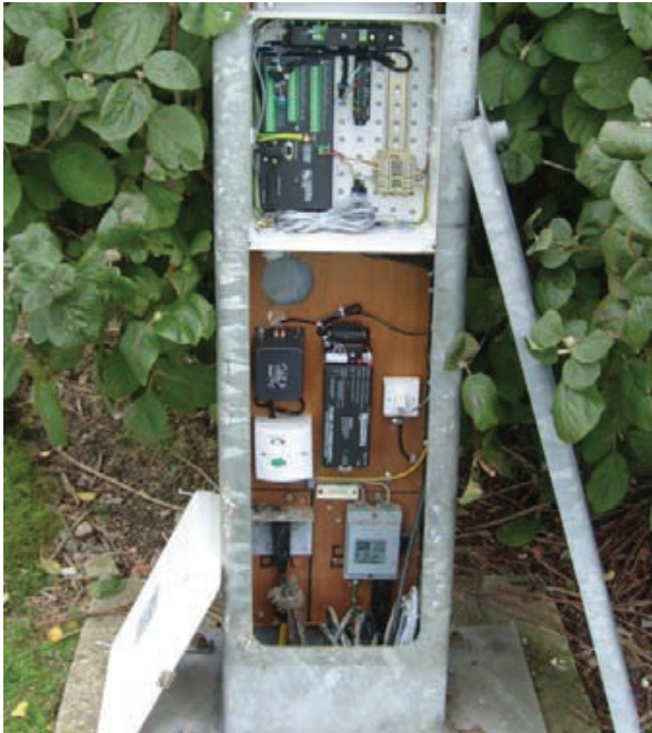
Above shows the instruments used in one of the AWS that monitors the Channel Tunnel.
