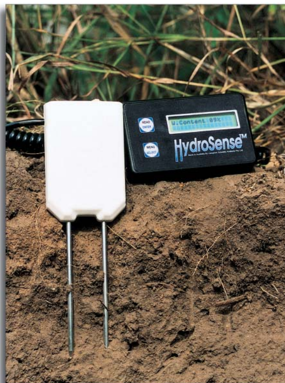
The portable HydroSense provides instant measurements, displayed as soil water content or water deficit.
