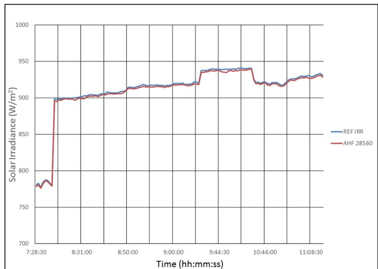
Figure 4. Comparison of Campbell Scientific’s AHF Cavity controller with the standard at NREL, Golden, Colorado.
