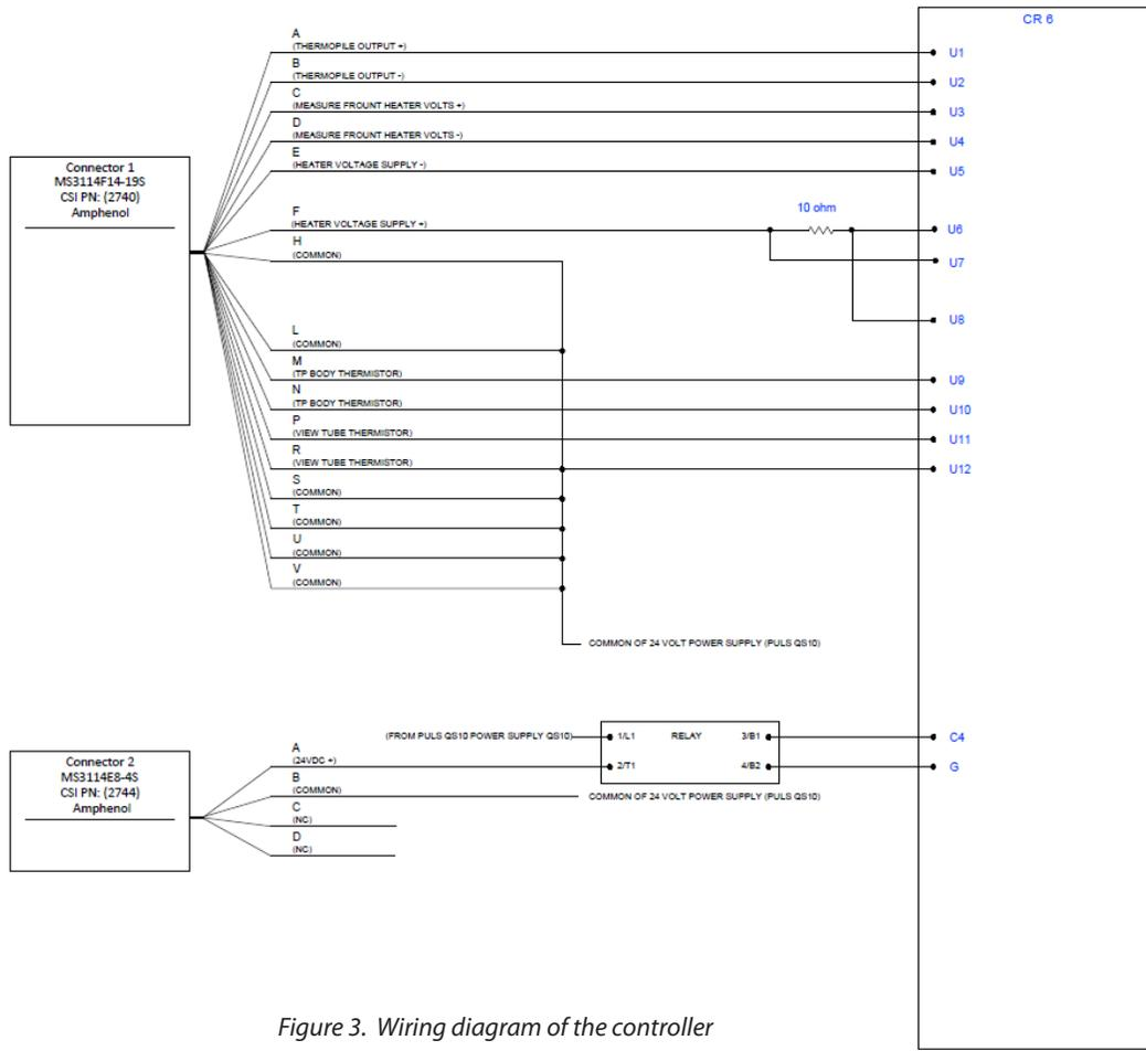
Figure 3. Wiring diagram of the controller
