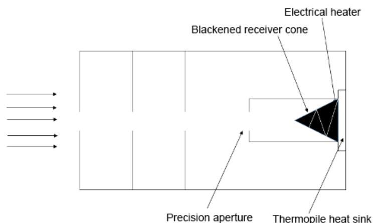
Figure 1. Schematic of a absolute cavity radiometer.
