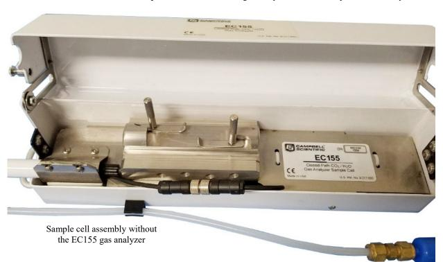
Step 7: Unscrew the bracket securing the sample intake tube.
