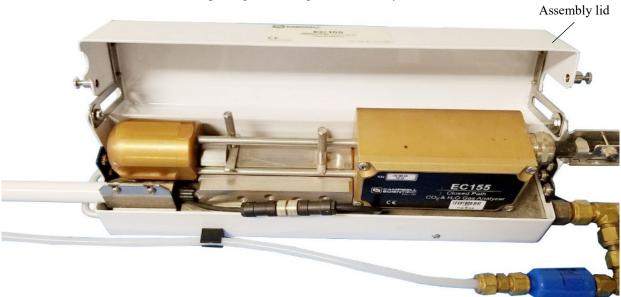
Step 3: Open the sample cell assembly lid.
