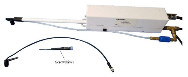
**Step 2:** Loosen spring-loaded screws on both sides of the sample cell assembly lid.
