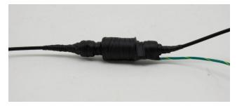
8. Extend the ground wire from the wrapping parallel to an antenna cable.
