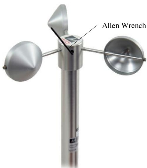
FIGURE 7-2. Allen wrench tightening bolt
