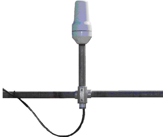
Figure 28: SAF5350A Antenna Mounted
