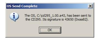
Once the download is complete, disconnect power from the CD295 for at least 30 seconds to ensure that it has been completely reset. After this, the new operating system will run.
