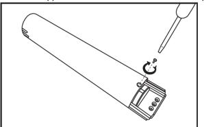
4. Install the 4-40 x 1/4 SS slot head screw supplied with the copper sleeve. Tighten the screw until snug. The hex screw is no longer needed.
