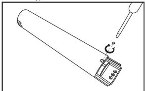
4. Install the 4-40 x 1/4 SS slot head screw supplied with the copper sleeve. Tighten the screw until snug. The hex screw is no longer needed.
