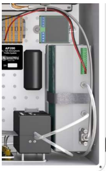
FIGURE 4-4. The IRGA installed in the AP200 system enclosure
