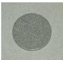
FIGURE 4-13. Disk filter of early AP200 intake assembly
