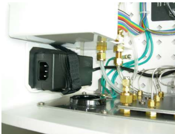
FIGURE 4-8. AC/DC power adapter kit installed in AP200
