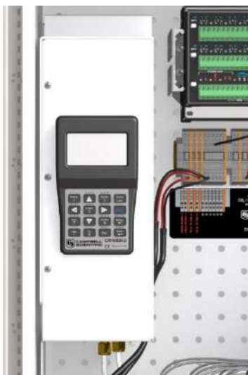
FIGURE 4-7. AP200 keyboard display mounted in system enclosure
