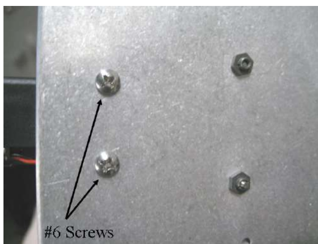
FIGURE J-8. Self-tapping screws attaching pump to metal box
