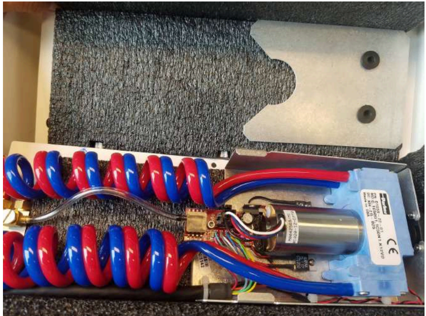
FIGURE J-12. Proper placement of AP200 pump (SN 33240) back into foam of pump enclosure.
