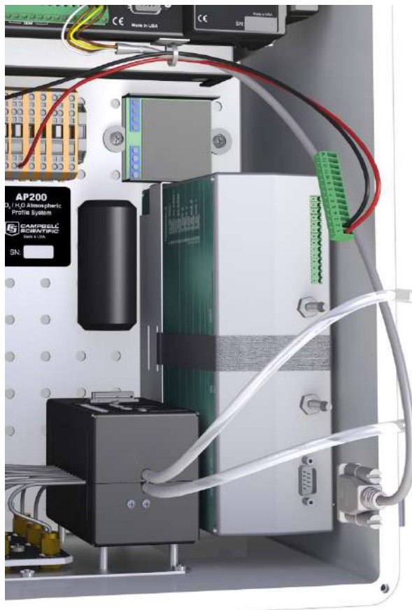
FIGURE 7-5. Components and fittings of IRGA installation
