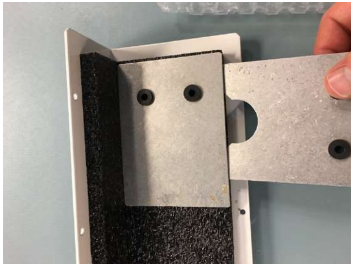
FIGURE J-4. Removal of original pump module inner plate and replacement with new inner plate provided in pump replacement kit (pn 33241)
