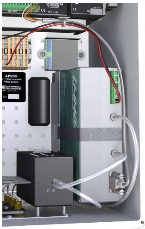
FIGURE 7-4. Installed IRGA in system enclosure
