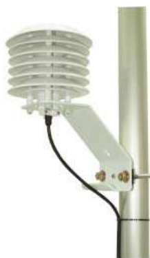
FIGURE 4-10. 107-L temperature probe mounted with radiation shield
