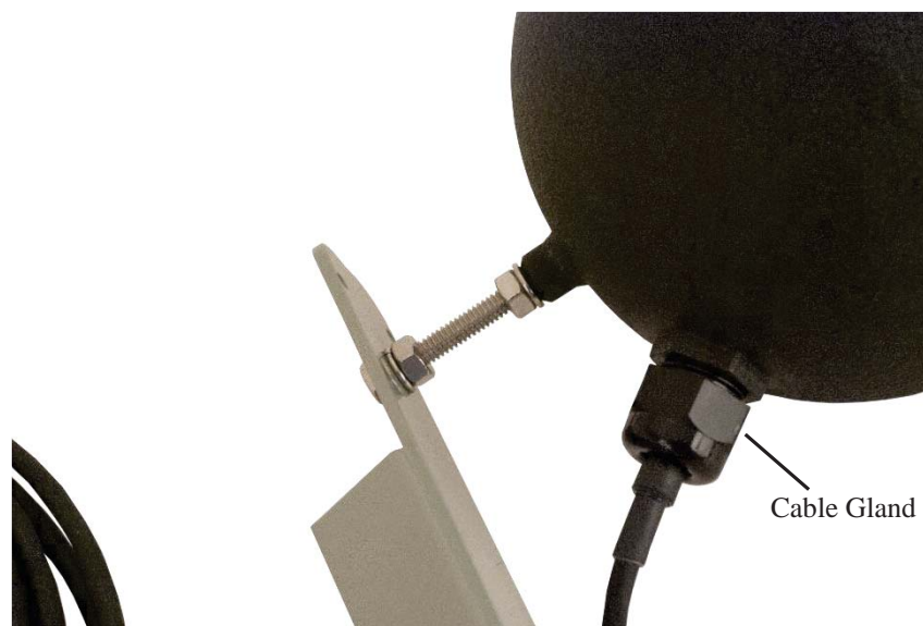
FIGURE 6-3. BlackGlobe fitting and cable alignment
