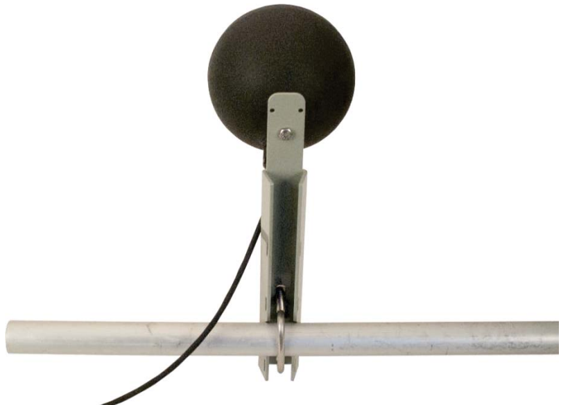
FIGURE 6-5. BlackGlobe mounted to a crossarm (back view)
