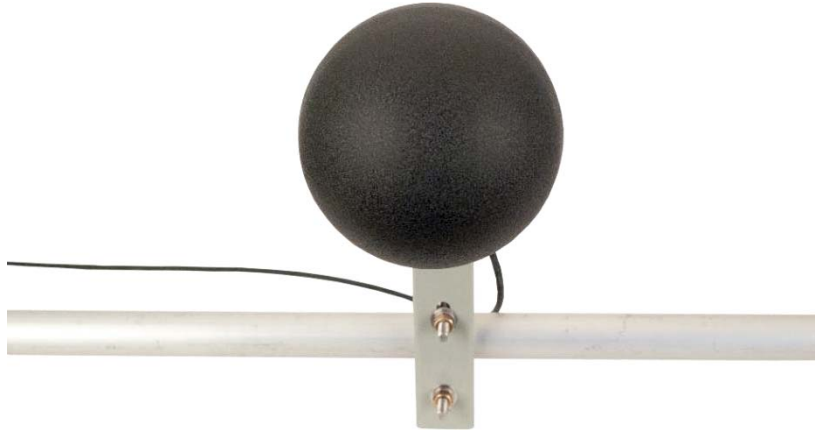
FIGURE 6-4. BlackGlobe mounted to a crossarm (front view)
