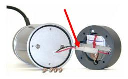
3. Remove the dessicant packs by undoing the twist tie that holds them in place and dispose of the packs appropriately.
