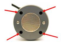
2. Remove the transducer housing from the main cylinder housing and unplug the white connector, as indicated below. Pull only on the connector and not the wires.
