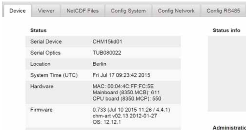
Fig. 12: Web interface device menu in standard user mode. The field is displayed as the first, and shows status information. A login as superuser or service user is available.
