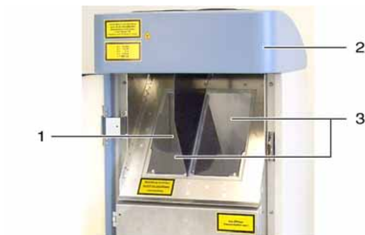
Fig. 26: Glass panels have to be cleaned
