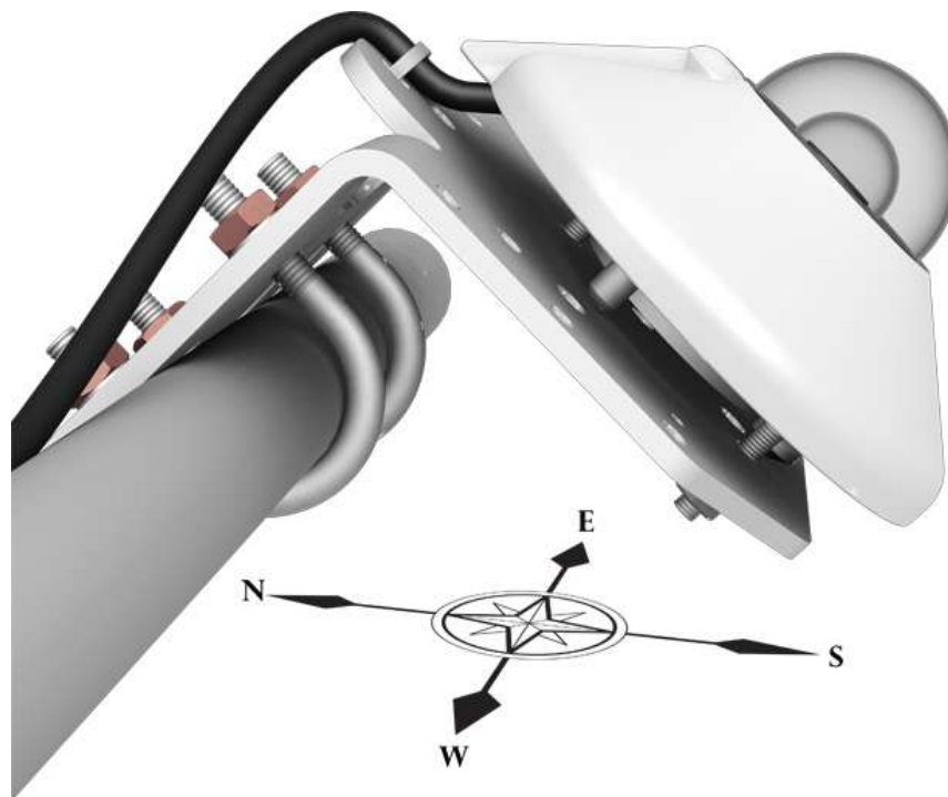
FIGURE 4-4. Pyranometer mounted at an angle for the Southern Hemisphere
