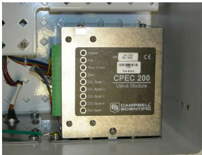
FIGURE 4-8. CPEC200 six-valve module (pn 26578)
