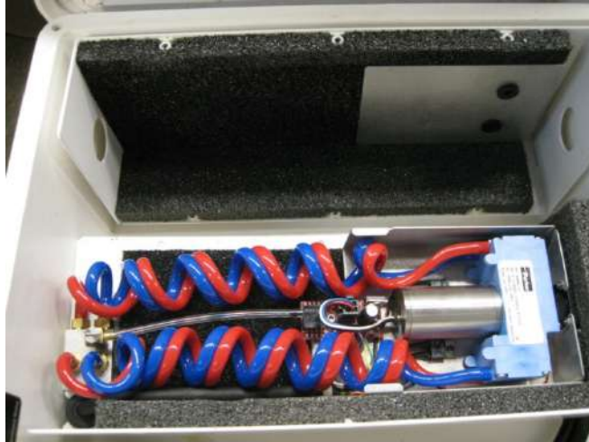
FIGURE H-4. Exposed CPEC200 pump assembly
