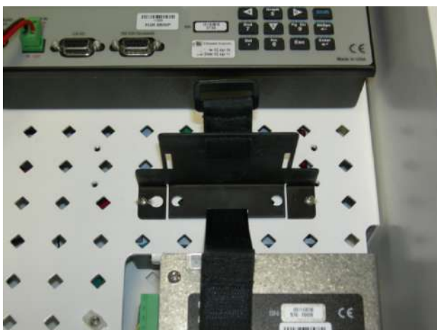
FIGURE F-1. Peripheral mounting kit installed in CPEC200 enclosure
