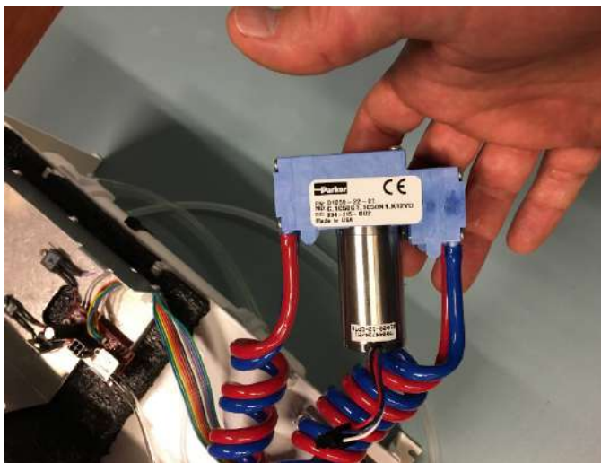
FIGURE H-11. Inlet and outlet tubing reconnected to pump
