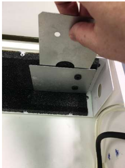
FIGURE H-5. Removal of original pump module inner plate and replacement with new inner plate provided in pump replacement kit (pn 33241)
