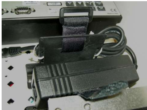
FIGURE F-2. Power supply in mounting bracket
