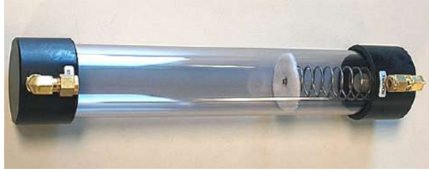
FIGURE G-4. Empty bottle showing the top (on the right with spring) and bottom (left) caps
