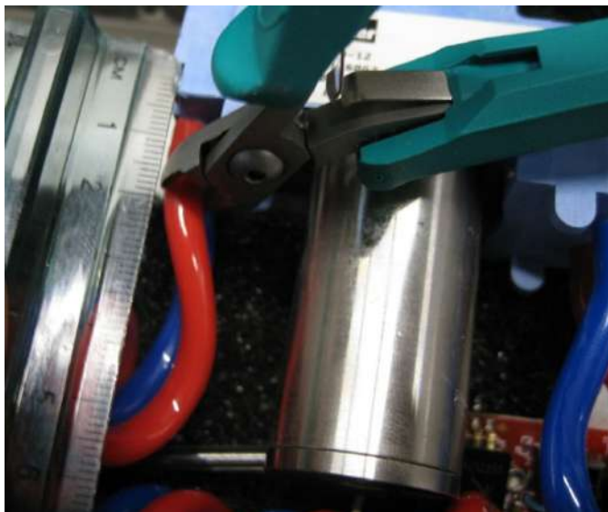
FIGURE H-10. Location of cuts to remove pump assembly from tubing
